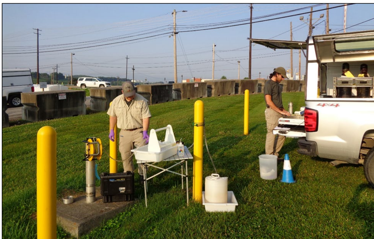
Figure 4.27. Groundwater monitoring well sampling in the Upper East Fork regime at Y-12
